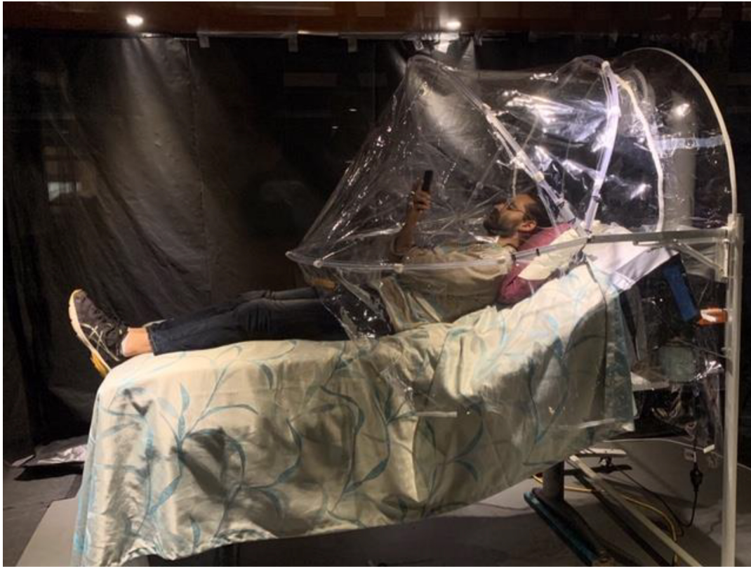
Figure 1. Photo of the personal protective ventilation hood*
